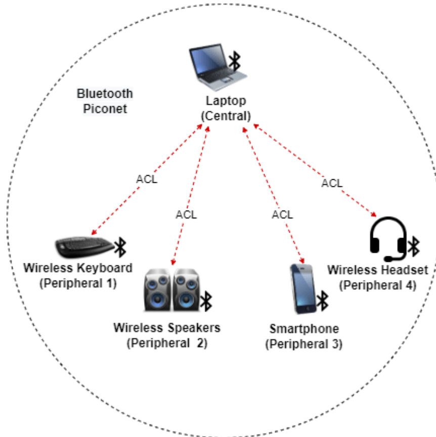
Simulation Scenario Showing Multiple Peripherals in a Bluetooth BR/EDR Piconet
