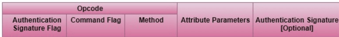
Service Data Unit - Attribute Protocol(ATT) PDU format
